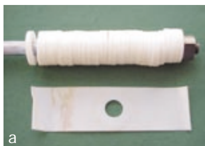
Fig 7. The same coupon rack as shown in Figure 6. The rouge deposits at the water line is very distinct.
