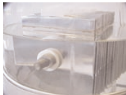
Fig 6. Test cell with a coupon rack showing rouge at the water line after 3 weeks exposure in WFI purged with N 2 (boiling was paused). The coupons include both the #80 and the 2B + ep finish of EN 1.4435 material.
