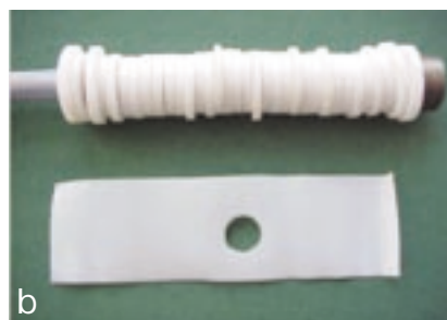
Fig 8. Teflon spacers and strips after exposure of EN 1.4435 in WFI purged with a) Air + 1% CO 2 and b) Air minus CO 2 .
