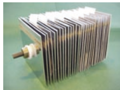
Fig 7. The same coupon rack as shown in Figure 6. The rouge deposits at the water line is very distinct.
