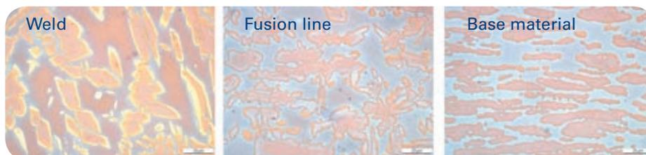
**Fig. 4** AL2003 6g, metallographic cross section of the weld (electrolytically etched with NaOH)
