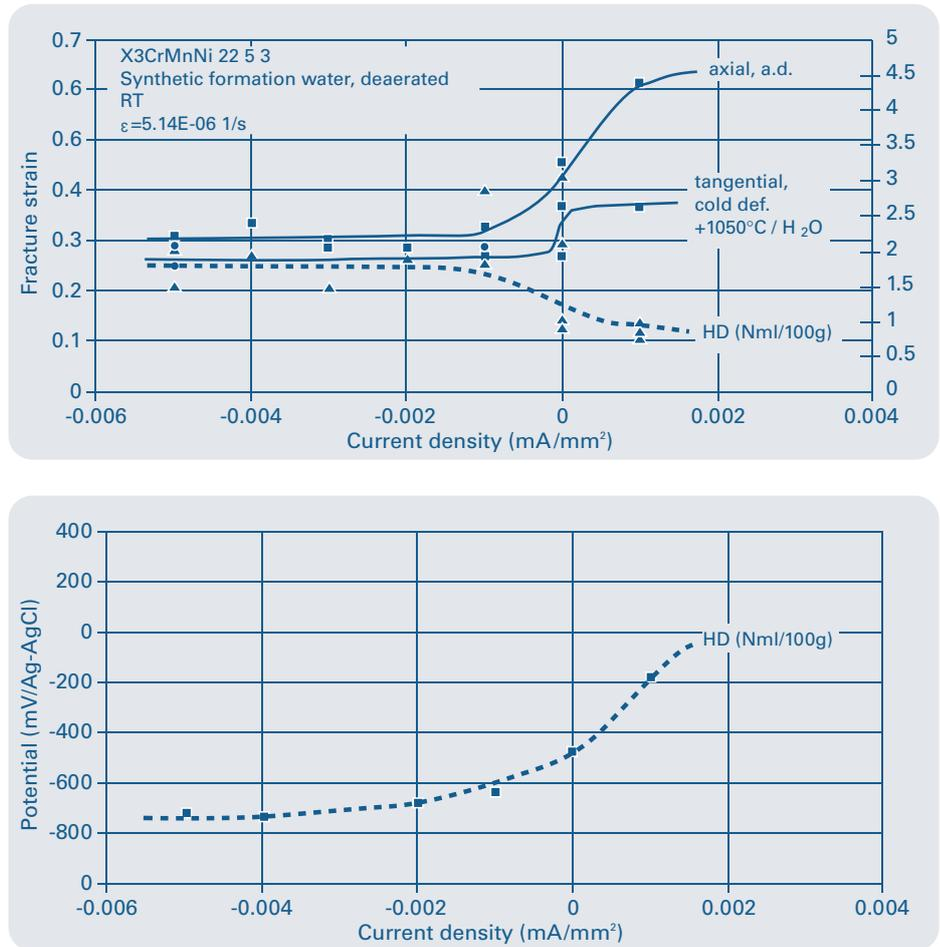
**Fig. 7** X3CrMnNi 22 5 2 fracture at  $\epsilon = 5.14 \text{ E-}06 \text{ 1/s}$
