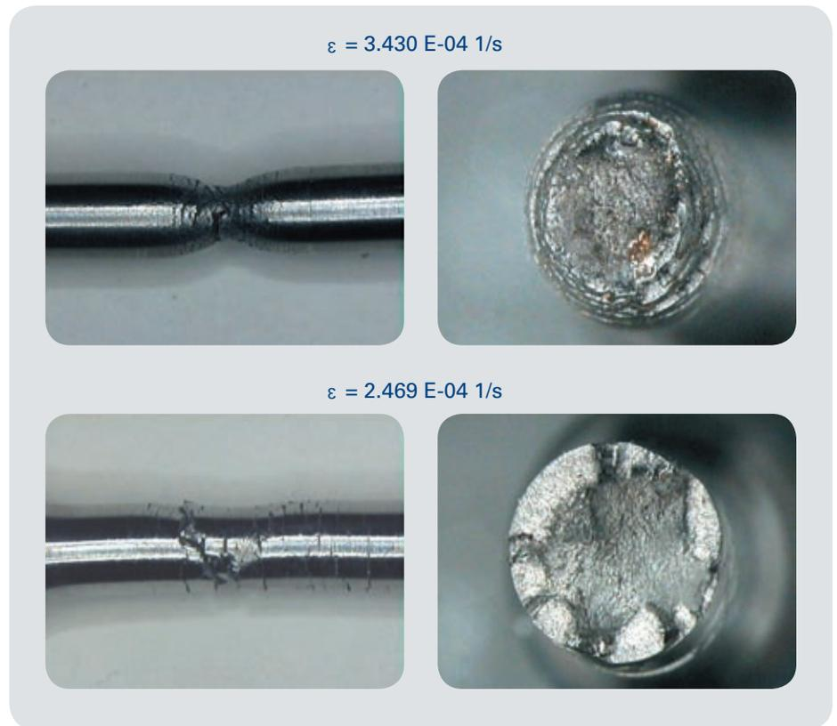
**Fig. 11** X6CrNiMo 12 6 2 fracture at  $i = - 0.0038 \text{ mA/mm}^2$
