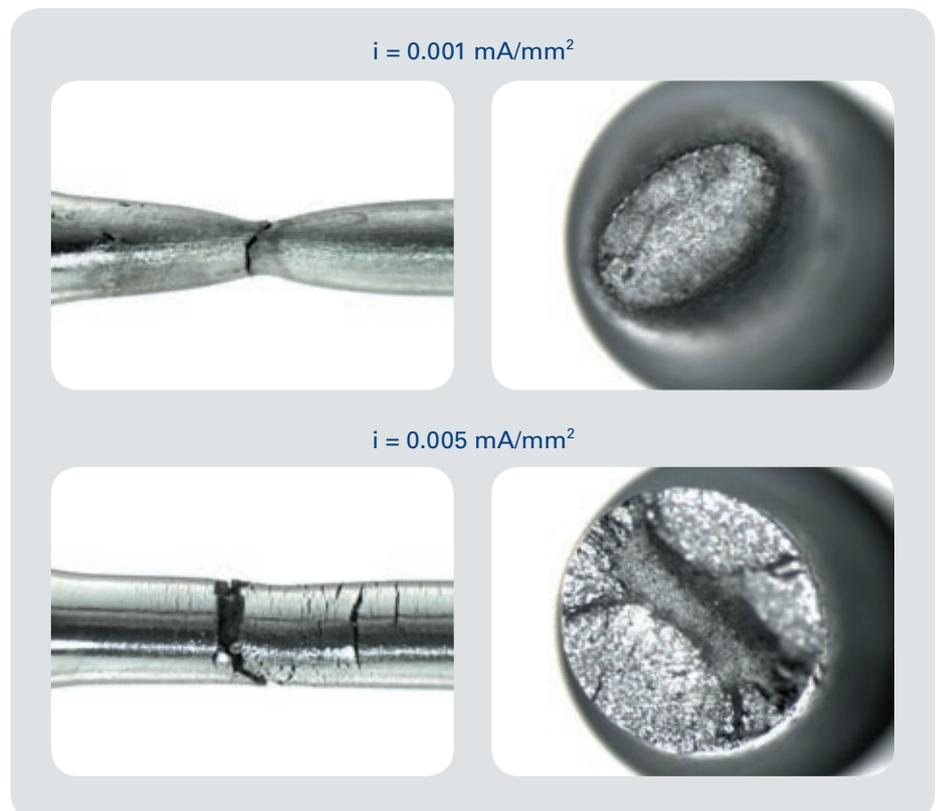
**Fig. 6** Effect of cathodic charging on diffusible hydrogen, fracture strain and potential of X3CrMnNi 22 5 2 at  $\epsilon = 5.14 \text{ E-}06 \text{ 1/s}$
