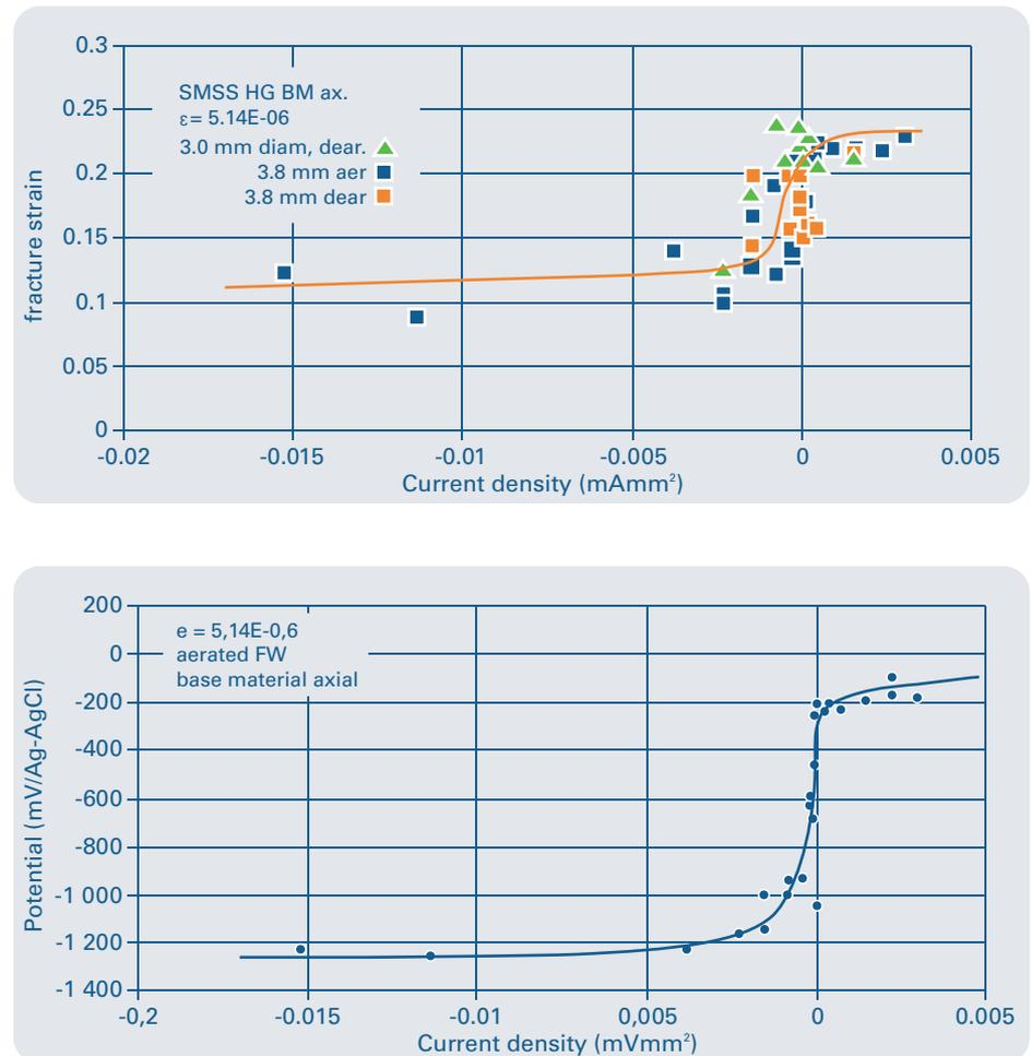
axial tensile ductility transition from anodic to cathodic conditions by reduction from a fracture strain of 0.25 to a plateau of about 0.1 at high cathodic current densities. At the same time the measured potentials drop from about -100 mV to -1200 mV. The SMSS thus loses about 60% of its original ductility in the axial to the pipe direction.
