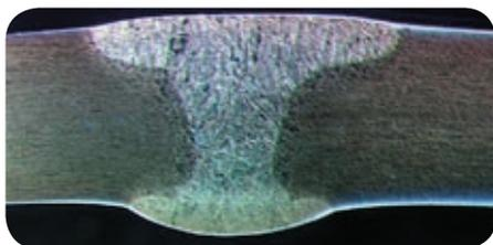
**Fig. 3** LDX 2101 6g, metallographic cross section of the weld (electrolytically etched with NaOH)
