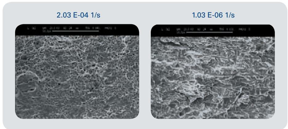
**Fig. 16** Secondary cracks in  $\delta$  and  $\gamma$  at  $-0.0038 \text{ mA/mm}^2$  after axial testing
