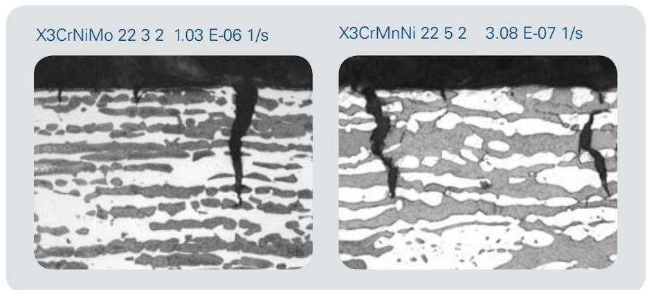
**Fig. 17** Microstructures in axial direction
