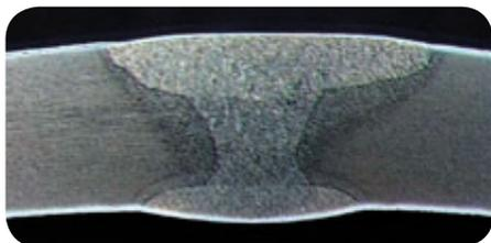
**Fig. 5** AL2003 6g, metallographic cross section of the weld (electrolytically etched with NaOH)
